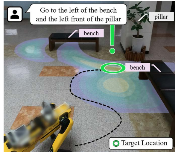
Figure 1: An illustration of incremental space grounding in the navigation task. Our method, LINGO-Space, identifies the distribution of the target location indicated by a natural language instruction with referring expressions.
