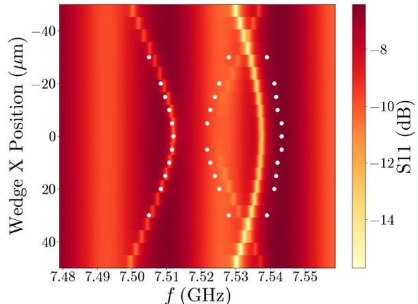
FIG. 4: Mode map showing the effects of misaligning the wedge in the X direction. Each row is an  $S_{11}$  sweep at a given wedge position. The measured resonant modes are visible as curved bright lines (the vertical bars are known VNA calibration artifacts). The resonant frequencies given by FEA, shifted down by 15.23 MHz, are overplotted as white points.
