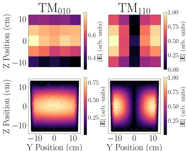
FIG. 3: The first column shows the  $TM_{010}$  mode mapped with a dielectric disk (top) and using eigenfrequency FEA using COMSOL-RF (bottom). The second column shows the same for the  $TM_{110}$  mode. The measured and simulated plots use independent  $|E|$  scales. For details on the field mapping procedure, see the main text Sec. III B. The agreement between the measured and simulated field maps aids in identifying the  $TM_{010}$  mode.
