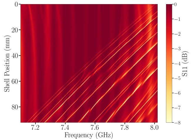
FIG. 2: Mode map showing the tuning range of the prototype cavity explored in this study. Each row is an S11 sweep at a given shell Z position. The measured resonant modes are visible as bright lines (the vertical ripples are known VNA artifacts). The axion-sensitive  $\text{TM}_{010}$  mode has the lowest frequency, and tunes uniformly from 7.1 GHz to 8 GHz. The wedge was aligned every 0.4 mm (3.9 MHz) using the procedure detailed in Sec. III C.
