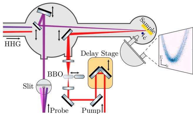
FIG. 2: The trARPES setup includes the pump-probe beamline of the VUV laser source and the integration with the HHG source ("Harmonium").
