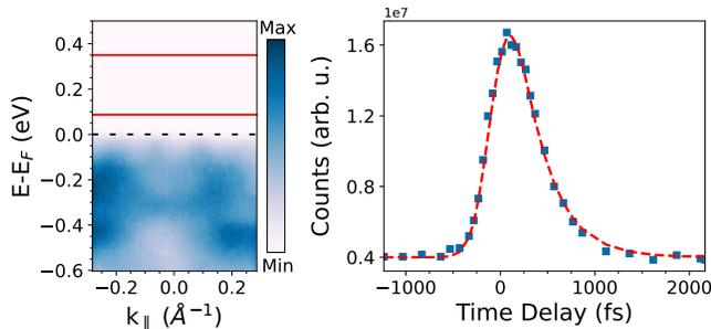
FIG. 6: Left: EDC of TaTe<sub>2</sub>. The red area marks the unoccupied region used to extract the time resolution from the time trace on the right. Right: Dynamics of the unoccupied region of TaTe<sub>2</sub> after pump excitation (blue), fitted with an exponential decay model according to Eq. 2 (red dashed line). The fit shows a time resolution of 410 fs. Measurement conditions:  $\hbar\omega = 10.8$  eV, slit = 500  $\mu\text{m}$ ,  $T = \text{RT}$ .
