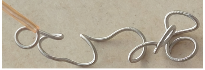
(b) Expulsion of an actual coil into regular surrounding (air) with contactless loop formation and curling
