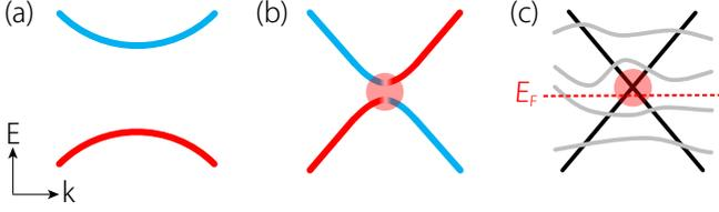
FIG. 1. (a) Well separated bands with relatively small quantum metric. The blue and red colors here represent different character of the states. (b) Quantum metric is pronounced at a band (anti-)crossing. (c) Such band (anti-)crossings around Fermi level act like hot spots for large quantum metric in a general band structure.
