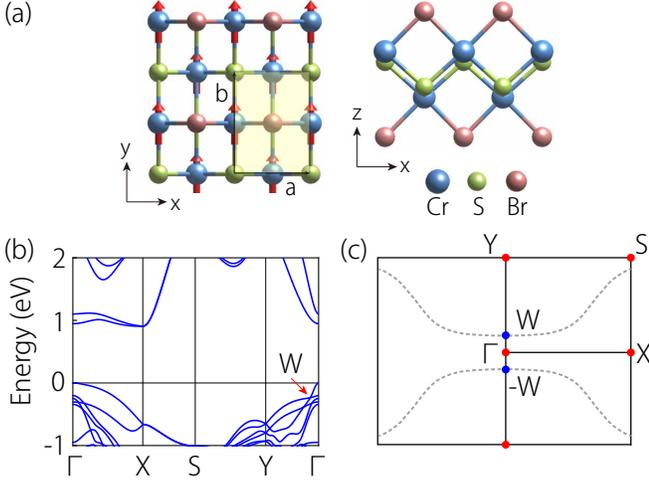
FIG. 3. (a) Top and side views of monolayer CrSBr. The shaded rectangle indicates the unit cell. The red arrows denote the local spins on Cr sites in ground state. (b) Calculated band structure of monolayer CrSBr. (c) Brillouin zone. The dashed lines indicate the two gaped nodal lines.  $\pm W$  are the two Weyl points.
