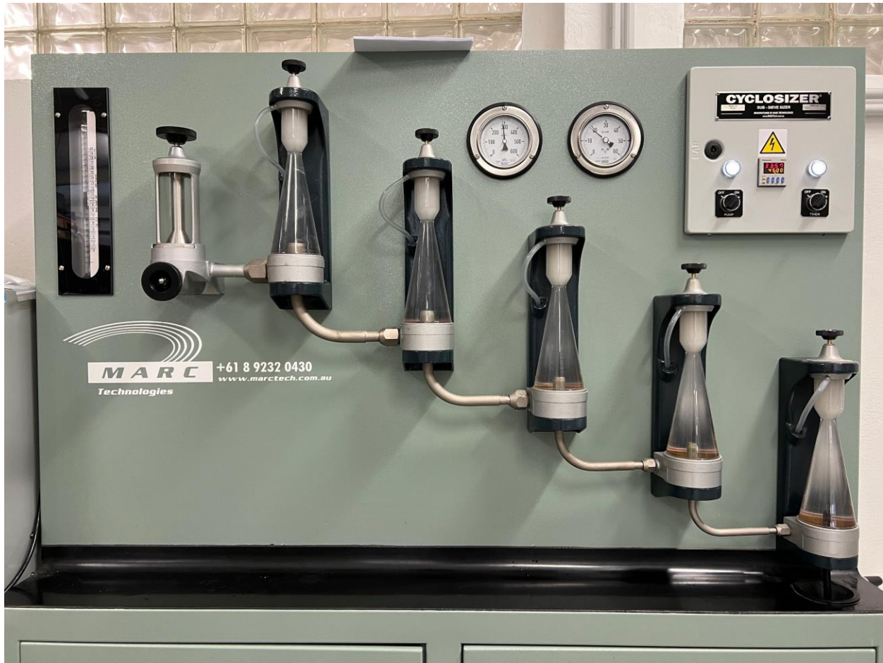
Figure 2. The Cyclosizer M16 with the 5 cyclones used for the separation tests of this study.
