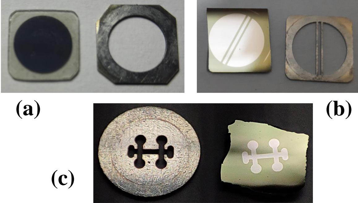
**Figure 2.4:** Deposited thin films and different stainless steel masks used for thin film deposition: (a) 8-*mm*-diameter *a*-MoGe thin film deposited on MgO substrate with the stainless steel mask, (b) 8-*mm*-diameter *a*-MoGe thin film grown in surface-oxidized Si substrate with strip lines for measuring the thickness with the mask, and (c) deposited hall-bar-patterned *a*-MoGe thin film with the mask. (Photo courtesy: Dr. Subhamita Sengupta).
