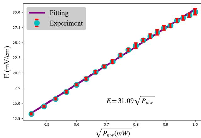
FIG. S2. **Calibration of the MW strength.** The actual strength of the target MW field is calibrated, and fit to be  $E(mV/cm) = 31.09\sqrt{P_{MW}}(mW)$ .
