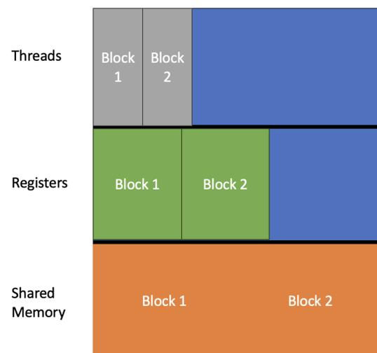
Figure 12: Data Parallel A100 SM Resource Usage
