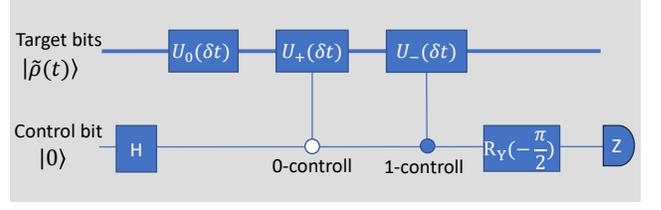
FIG. 2. Illustration of quantum circuit for the temporal propagation of DQME-SQ within a single time step by utilizing the LCU algorithm.
