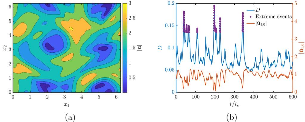
Figure 4: (a) The instantaneous velocity amplitude  $|\mathbf{u}|$  for the Kolmogorov flow. (b) Time history of  $D(t)$  and  $|\check{\mathbf{u}}_{1,0}(t)$  for  $\eta = \bar{D} + 1.5\sigma_D$ .
