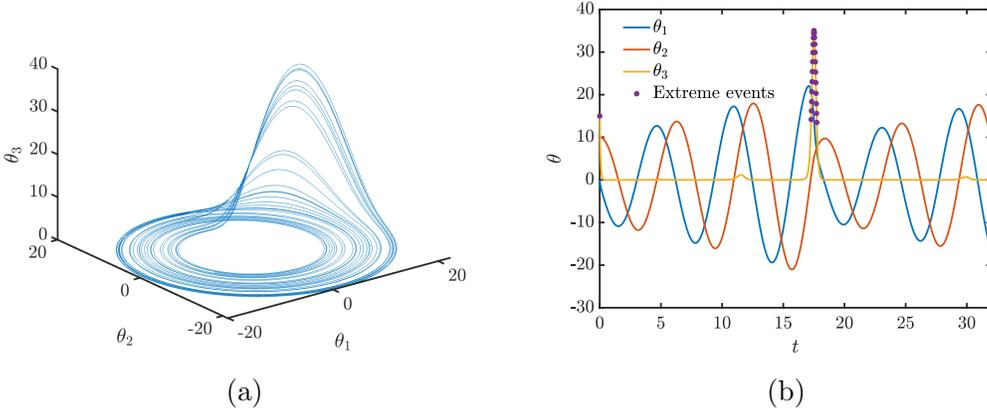
Figure 1: (a) Trajectory of the Rössler system. (b) Extraction of time series of  $\theta_1$ ,  $\theta_2$ ,  $\theta_3$  and extreme events in the Rössler system. Although not shown, the whole time-span of the signals is 10,000 time units.
