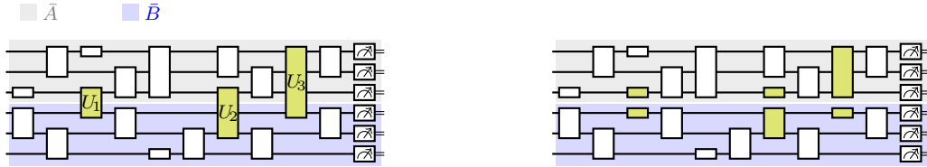
Figure 5: Circuit Cutting Example. The circuit on the left has 3 gates which cross a partition of the qubits into 2 clusters, \bar{A} and \bar{B} , indicated by the background colors. Using a quasi-probability decomposition of each gate, it becomes possible to express the output of the circuit on the left as a sum of outputs of circuits having the form on the right, where each of the indicated gates is replaced gates which act locally on qubits in each cluster. The total number of circuits needed (the sampling overhead depends on specific properties of each gate being cut, along with the particular details of the cutting method used. NOTE: Image is taken from [339], and is used with permission.
