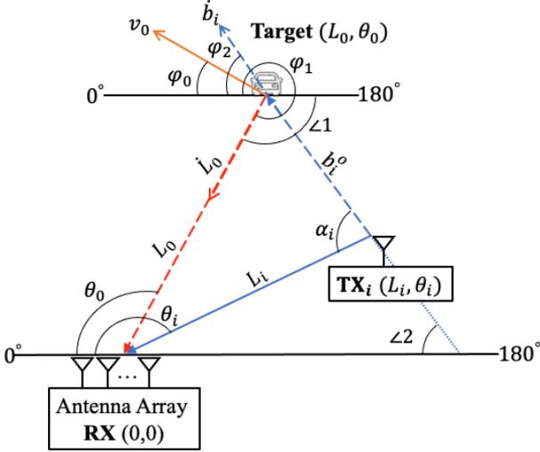
Fig. 3. Velocity projection when  $\theta_0 < \theta_i$ .
