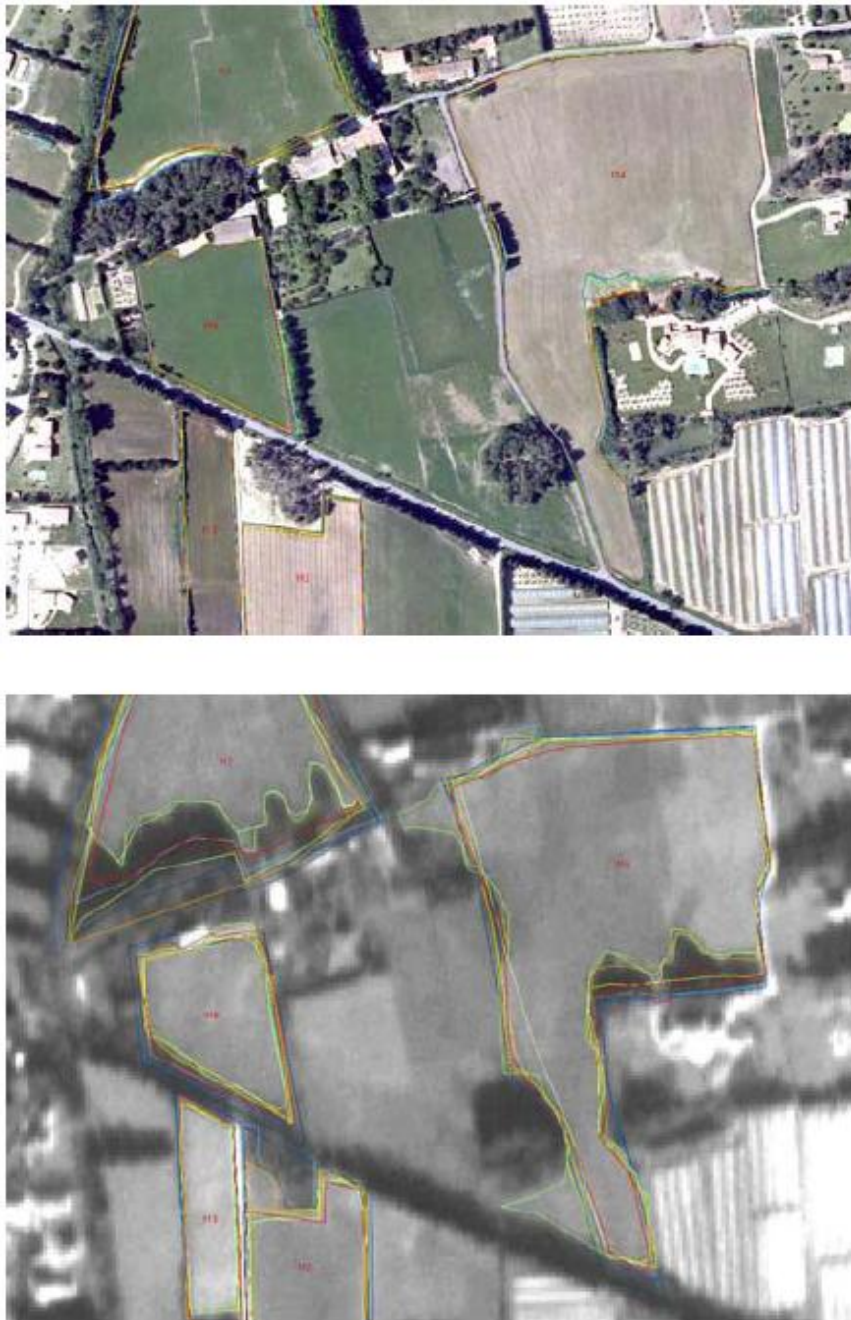
Figure 3. Example of area measurement on orthophoto and Cartosat1 images
