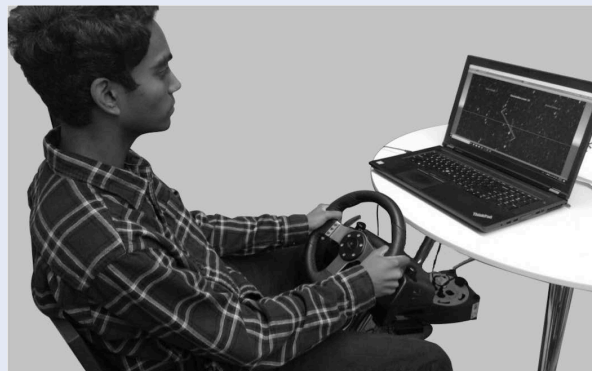
FIGURE S2: Bumps are added using a motor torque in the wheel. Experiments can be done with bumps only or trails only, or both together, and with varying trail speed and/or advanced-warning, and with additional quantization and/or time delay in the map from wheel position to players' actual position.
