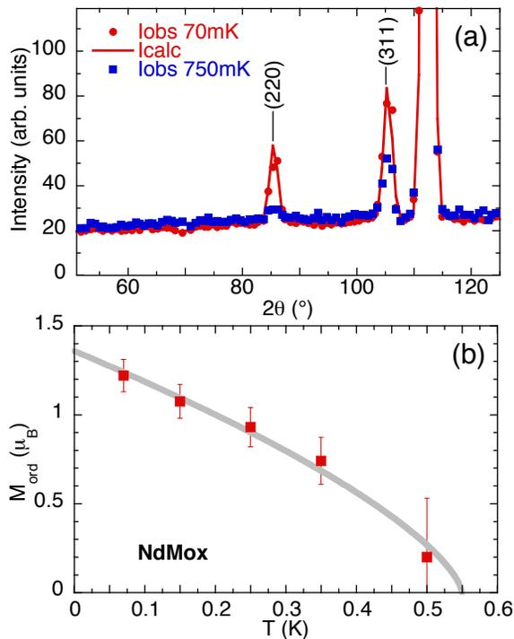
FIG. 6. (a) Neutron diffractogram measured for NdMox by integrating the inelastic data measured on FOCUS between  $-0.1$  and  $0.1$  meV at 70 mK (red dots) and 750 mK (blue squares). The red line is a refinement to an all-in-all-out magnetic structure. (b) Ordered magnetic moment as a function of temperature determined from the diffractogram. The line is a guide to the eye.
