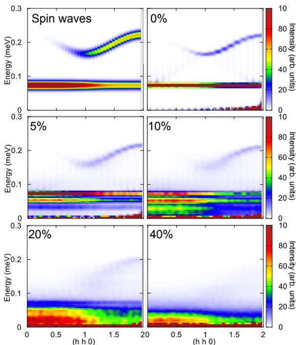
FIG. 13. Calculated inelastic neutron scattering spectra along  $(hh0)$  at zero temperature and for different substitution rates. The top left figure shows the spin wave calculations, to be compared with the 0 % calculations.
