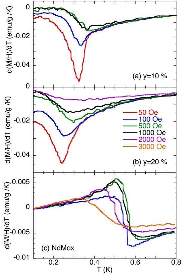
FIG. 18. Derivative of  $M/H$  with respect to the temperature in  $(\text{Nd}_{1-y}\text{La}_y)_2\text{Zr}_2\text{O}_7$  with (a)  $y = 10\%$ , (b)  $y = 20\%$  and in (c) NdMox for several applied fields between 50 and 3000 Oe.
