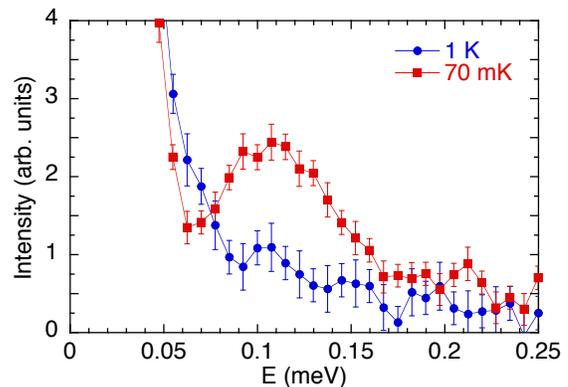
FIG. 9. Energy scan in NdMox measured on FOCUS at 70 mK (red squares) and 1 K (blue dots), in which the signal has been integrated over the  $Q$ -range  $[0.5; 1.6]$  Å $^{-1}$ .
