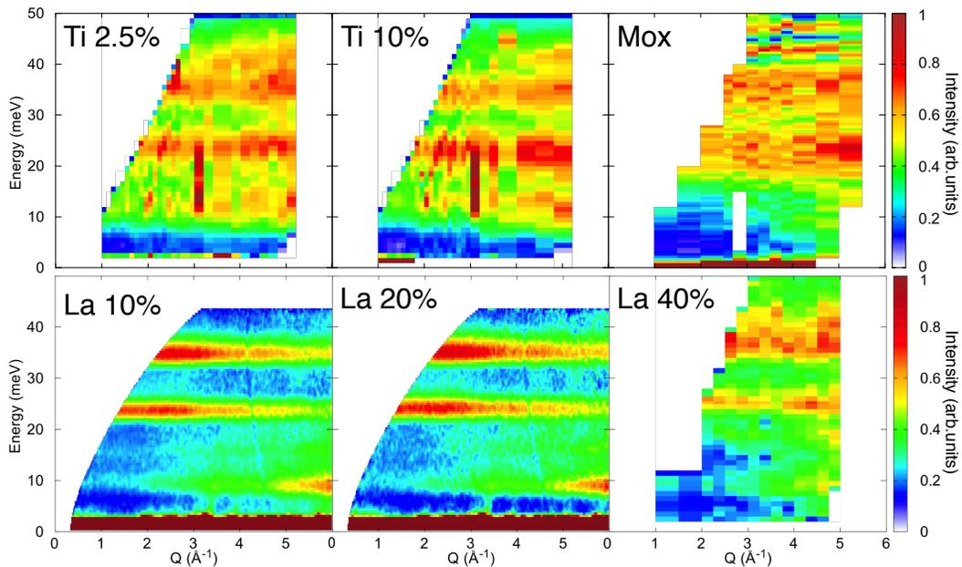
FIG. 2. Inelastic neutron scattering spectra at  $T = 3.8$  K in  $\text{Nd}_2(\text{Zr}_{1-x}\text{Ti}_x)_2\text{O}_7$  with  $x = 2.5$  and 10 % measured on 2T, and at  $T = 1.5 - 1.6$  K for  $(\text{Nd}_{1-y}\text{La}_y)_2\text{Zr}_2\text{O}_7$  with  $y = 10$  and 20 % measured on PANTHER and  $\text{Nd}_2(\text{TiZrHfScNb})_2\text{O}_7$  and  $(\text{Nd}_{1-y}\text{La}_y)_2\text{Zr}_2\text{O}_7$  with  $y=40$  % measured on EIGER.  $Q$ -cuts of these spectra are shown in Appendix A.
