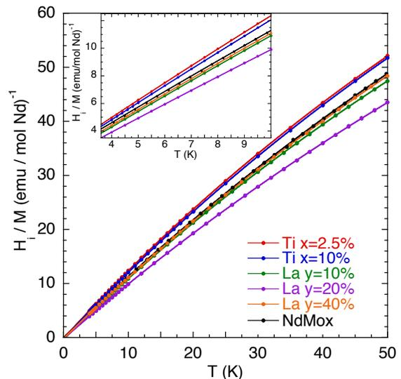
FIG. 3. Inverse approximate susceptibility  $H_i/M$  vs temperature  $T$  between 4 and 50 K with an applied field  $H \approx 1000$  Oe, where  $H_i$  is the internal field obtained after demagnetization corrections. The inset shows a zoom in these curves between 4 and 10 K. Lines correspond to fits using a Curie-Weiss law with a Van Vleck component. The resulting Curie-Weiss temperatures and effective moments are summarized in Table I.
