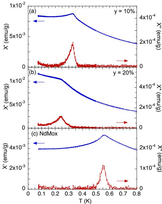
FIG. 4. AC susceptibility, in-phase  $\chi'$  (blue, left) and out-of-phase  $\chi''$  (red, right), as a function of temperature measured with an applied field  $H_{ac} = 1.8$  Oe and  $f = 0.57$  Hz for  $(\text{Nd}_{1-y}\text{La}_y)_2\text{Zr}_2\text{O}_7$  with (a)  $y = 10\%$ , (b)  $y = 20\%$  and for (c) NdMox.
