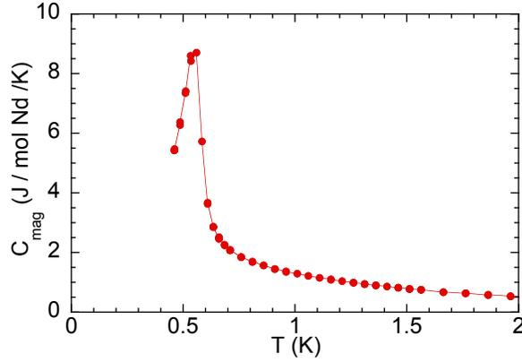
FIG. 17. Magnetic contribution to the specific heat  $C$  vs temperature  $T$  measured in NdMox. The YMox specific heat was subtracted from the raw data after a correction due to the different molecular weights [49].
