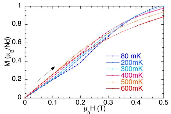
FIG. 11.  $M$  versus  $H$  at several temperatures in NdMox. The sample was first “saturated” in -1 T and the field was ramped up to 1 T.
