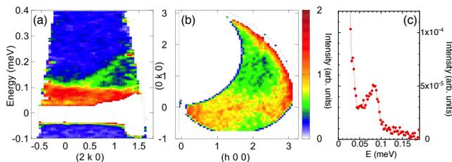
FIG. 7. Low energy excitations measured on  $\text{Nd}_2(\text{Zr}_{1-x}\text{Ti}_x)_2\text{O}_7$  with  $x = 10\%$  at 50 mK on IN5. (a) Spectra along  $(2k0)$  showing the flat mode and the dispersive branches measured with  $\lambda = 6$  Å. (b) Energy cut at  $E = 70 \pm 0.05$   $\mu\text{eV}$  showing the broadened pinch points measured with  $\lambda = 8$  Å. (c)  $Q$ -cut measured with  $\lambda = 10$  Å showing the persistence of a gap in the excitations.
