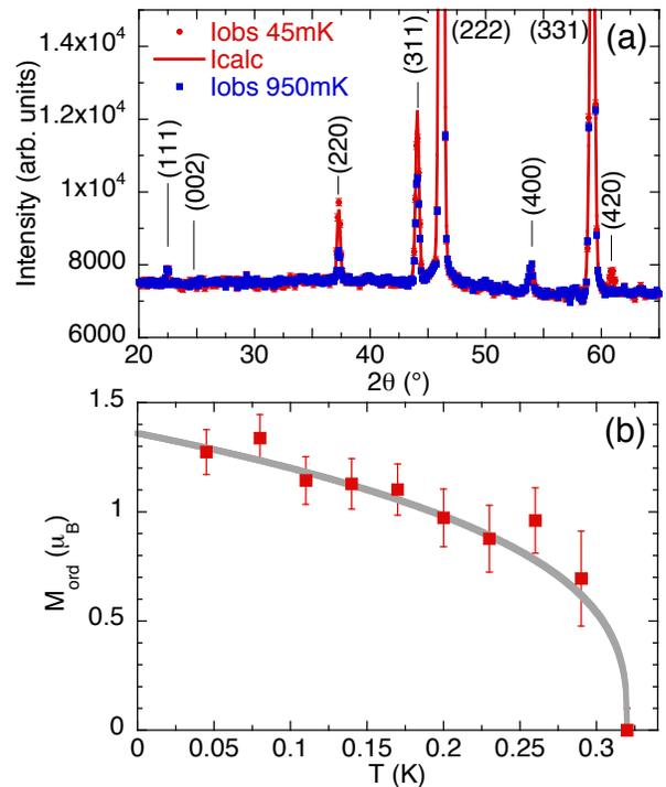
FIG. 5. (a) Neutron diffractogram measured on G4.1 for  $(\text{Nd}_{1-y}\text{La}_y)_2\text{Zr}_2\text{O}_7$  with  $y = 10\%$  at 45 mK (red dots) and 950 mK (blue squares). The red line is a refinement to an all-in-all-out magnetic structure. (b) Ordered magnetic moment as a function of temperature determined from the diffractogram. The line is a guide to the eye.
