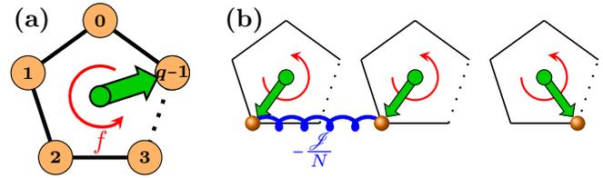
FIG. 1. (a) Potts spin (green arrow) with  $q$  states (orange bullets), driven by a non-conservative force  $f$  (red arrow). (b) The energy of interacting Potts spins is reduced by  $J/N$  whenever two spins are aligned.
