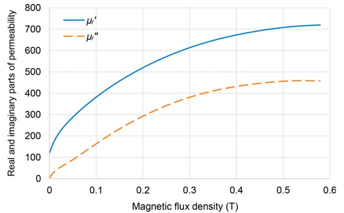
Fig. 2. Complex relative permeability for a LG steel.
