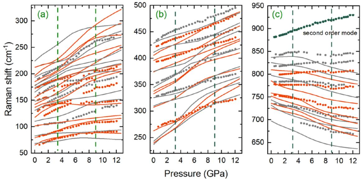
**FIG. 10.** Pressure dependence of experimental (symbols) and theoretical (lines) Raman-active modes of Zn(IO<sub>3</sub>)<sub>2</sub>. A tentative mode assignment of the experimental data is shown with different colors: Red and gray colors are used for A and B modes, respectively. In (c), we shifted all calculated modes by +70 cm<sup>-1</sup>, in order to facilitate the comparison with experiments.
