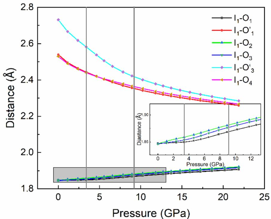
**FIG. 7.** Pressure dependence of the theoretical I-O bond distances. The inset shows a zoom of the I-O<sub>1</sub>, I-O<sub>2</sub> and I-O<sub>3</sub> distances below 13 GPa.
