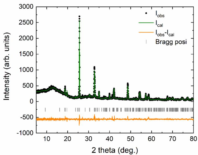
**FIG. 2.** XRD pattern measured at ambient pressure (circles). The green line is the Rietveld refinement. The quality factors of Rietveld refinement are  $R_p = 7.22\%$  and  $R_{wp} = 9.91\%$ . Residuals are shown in orange.
