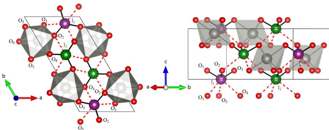
**FIG. 1.** Crystal structure of Zn(IO<sub>3</sub>)<sub>2</sub> at ambient conditions. (a) perpendicular to the c axis and (b) along the c axis. I atoms are shown in purple (I<sub>1</sub>) and green (I<sub>2</sub>) color. The Zn coordination octahedra are shown in gray. O atoms are shown in red and have been labeled. First neighbor I-O bonds are shown with solid black lines and second neighbor I-O bonds are shown with red dashed lines.
