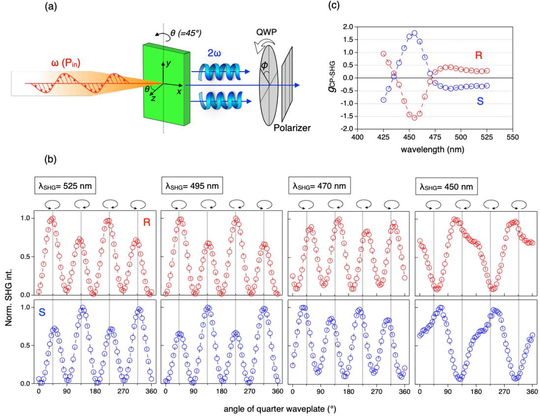
**Figure 4,** (a) Schematic representation of setup for detection of CP-SHG signal. The polarizer is placed on the detection side with cross polarizing to incident laser polarization. (b) The CP-SHG plot as function of angle of QWP of R (red) and S (blue) at several SHG wavelength. (c) The  $g_{CP-SHG}$  spectrum of R (red) and S (blue)
