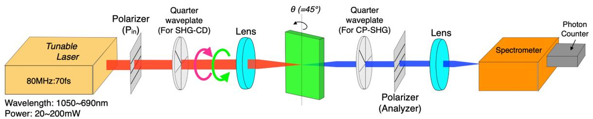
**Figure S2**, Schematic representation of optical se-up for SHG-CD and CP-SHG measurement
