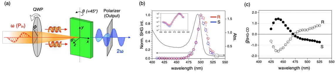
**Figure 2,** (a) Schematic of the experimental setup for SHG. (b) Normalized SHG intensity spectra of R- (red) and S-sample (blue) films, together with the UV-VIS absorption spectrum of the S-sample film. The inset in (b) shows the SHG spectra plotted on a log scale. (c) Spectra of the dissymmetric factors,  $g_{SHG-CD}$ , for SHG-CD without an output polarizer.
