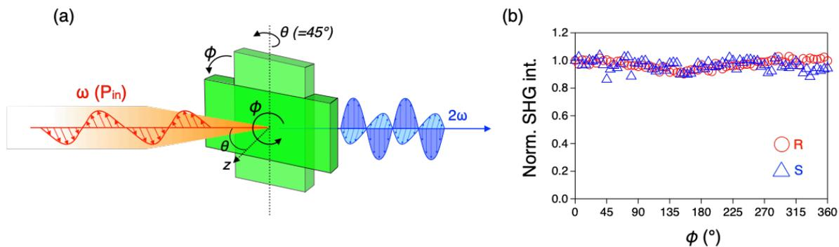
**Figure S4**, (a) Schematic representation of in-plane anisotropy measurement. While rotating the sample in-plane, SHG is recorded. (b) Normalized SHG intensity of R-/S-samples as function of in-plane sample rotation angle upon the stimulation of 990nm laser source.
