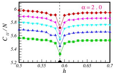
FIG. 4. (color online). The  $l_1$ -norm of coherence with respect to the magnetic field. The TSI is selected at  $\alpha = 2.0$ . Results are presented for chain sizes  $N = 600, 700, 800, 900$ , and  $1000$  from bottom to top.
