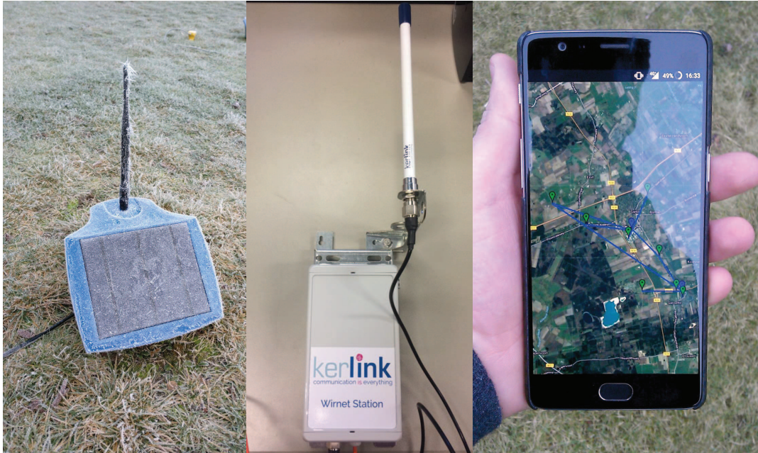
Fig. 13. On the left, LoRa-enabled with solar panel on top in freezing temperature of December; in the middle, Kerlink Wirnet Station providing direct 3G/4G connection as well as Ethernet connection possibilities, GPS with sub-meter location and microsecond time accuracies, and power on Ethernet (PoE) power supply; on the right, application tool running on a cell-phone providing real-time visual QC and status information.
