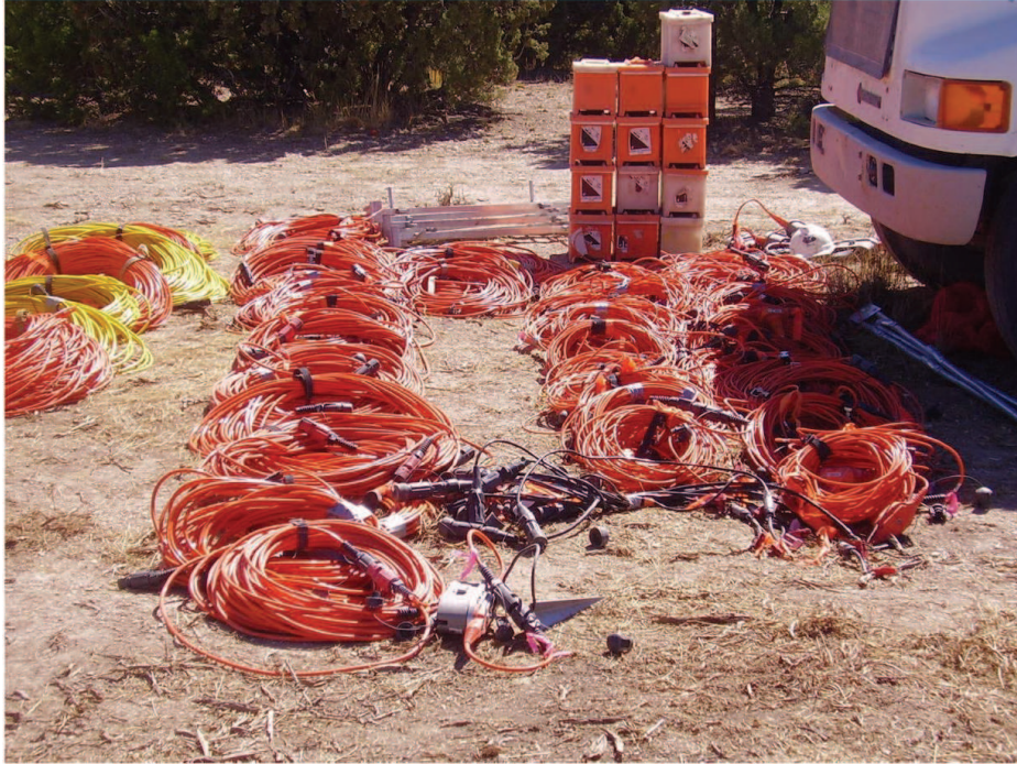
Fig. 4. Traditional cable-based seismic acquisition with tens of thousands of nodes connected through cables Kendall (2015).
