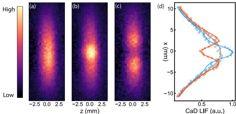
FIG. 2. Molecular-beam profile with Sisyphus cooling and heating. (a)–(c) Beam images under unperturbed, Sisyphus cooling at +40 MHz, and Sisyphus heating at –40 MHz configurations, respectively. (d) Integrated 1D profile. Sisyphus cooling narrows the width of the center of the molecular beam (blue), while Sisyphus heating expels molecules away from the center (red). Unperturbed beam is shown as gray. Solid lines show the fits to the beam profile.
