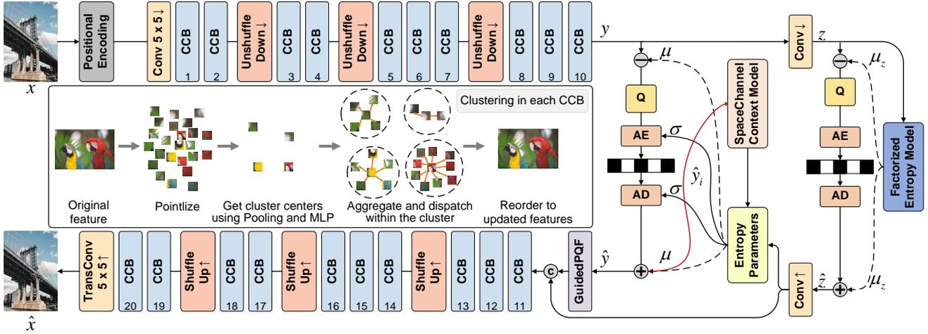
Figure 2: The overall architecture of the proposed method.  $\downarrow/\uparrow$  indicates downsampling/upsampling operations. The hyper encoder and decoder each consist of five convolutional layers, succeeded by a GELU function, except for the final layer. The channel of  $z$  is 192. Three hyper decoders are utilized for the mean, scale, and latent feature, respectively.
