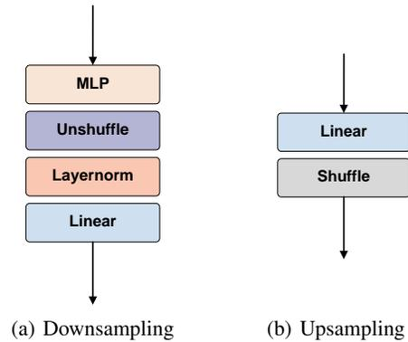
Figure 3: Structure of Down / Up sampling
