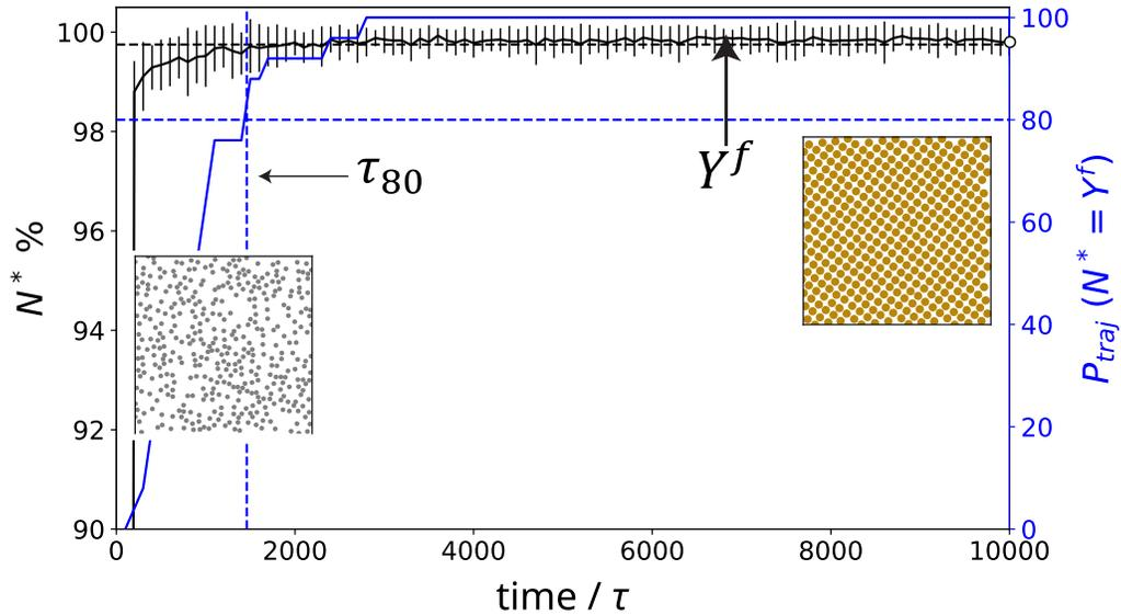
FIG. S6. **Self-assembly under the SQ NMO potential at the density  $\rho_{\text{SQ}} = 1$ .** Ensemble-averaged self-assembly trajectories showing the size of the largest contiguous cluster,  $N^*$  (black curve), and the fraction of trajectories that have reached  $Y_{\text{NMO}}^f = 99.75\%$ . Insets show representative snapshots of the initial and final configurations.
