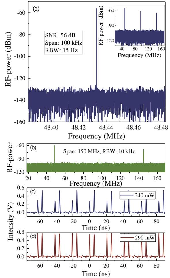
Fig. 4. (a) RF spectra of solitons states and soliton molecule states. (b) RF spectra of multi-pulse states, with intensity unit in dBm and SNR of the repetition rate at 59 dB. (c) Oscilloscope trace of multi-pulses at 340 mW. (d) Oscilloscope trace of multi-pulses at 290 mW.
