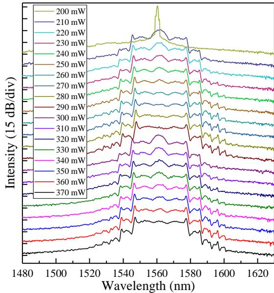
Fig. 5. Optical spectra of multi-pulse states operating at different pumping powers. The spectral bases are 15 dB apart.
