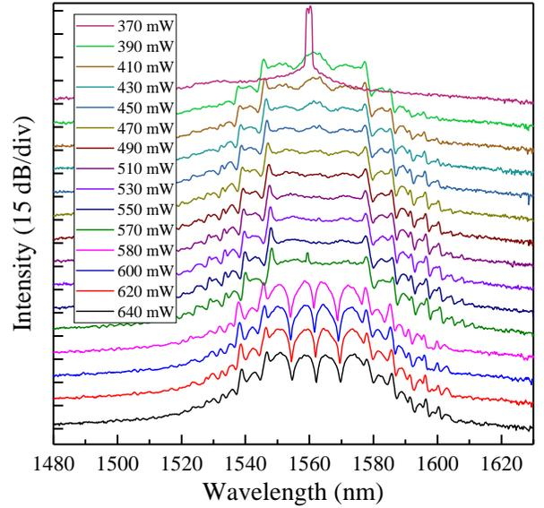
Fig. 3. Optical spectra of soliton states and soliton molecule states operating at different pumping powers. The spectral bases are 15 dB apart.
