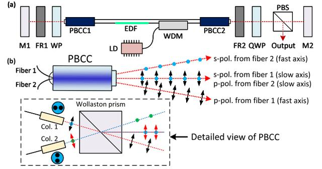
Fig. 1. (a) Experimental setup of the mode-locked fiber laser with a linear shape. M1 and M2, Mirror; WP, wave plate; EDF, erbium-doped fiber; WDM, wavelength division multiplexer; FR1 and FR2, Faraday rotator; LD, 976 nm laser diode; PBCC1 and PBCC2, polarization beam combiner collimator; PBS, polarizing beamsplitter. (b) The schematic of the polarization beam combiner collimator. Col. 1 and Col. 2, collimators; s-pol. and p-pol., s-polarized and p-polarized lights.
