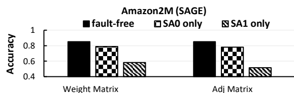
Fig.3. The accuracy of trained model after introducing 5% SA0 or SA1 pre-deployment faults on the weight and adjacency matrix separately.
