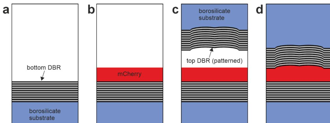
**Figure S2.** Schematic representation of the sample assembly. Starting with a planar DBR consisting of alternating SiO<sub>2</sub>/TiO<sub>2</sub> layers (a), a solution of mCherry in water is pipetted on top and spread (b). Finally, the second, patterned DBR (c) is applied to the mCherry (d), pressed and left to dry under constant pressure for 48 hours.
