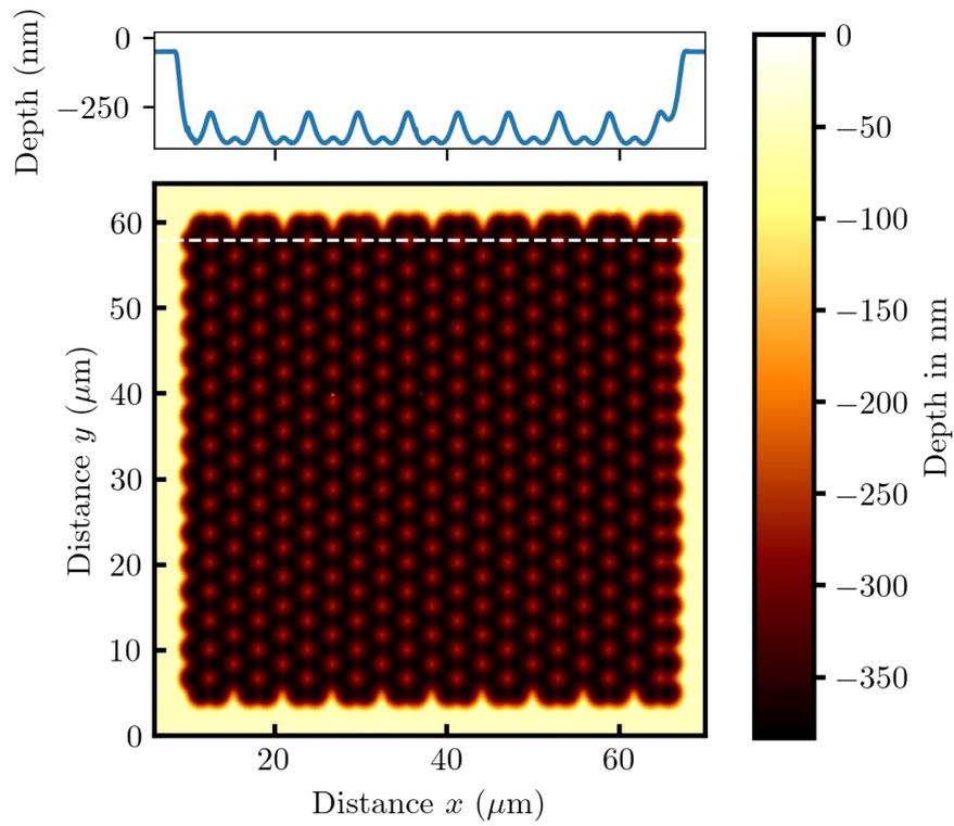
**Figure S1.** Visualization of the photonic potential landscape illustrated by an AFM image of the honeycomb lattice. The sites have a diameter of  $4 \mu\text{m}$ , a depth of about  $380 \text{ nm}$  and a center-to-center distance of  $2 \mu\text{m}$ .
