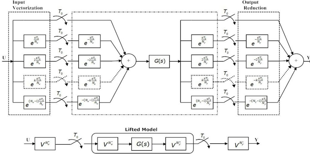
Figure 5: Kranc vector switch decomposition. General case
