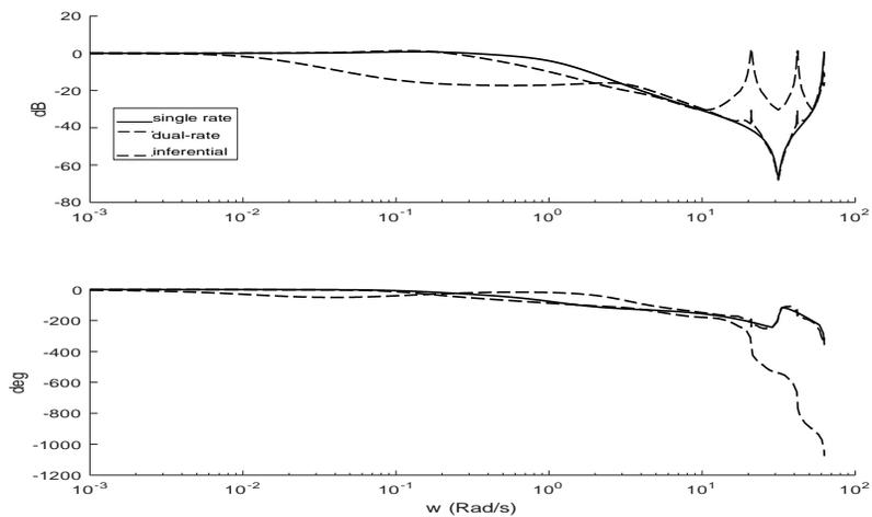
Figure 12: Example 1. Y/R DR systems Bode. Methods comparison
