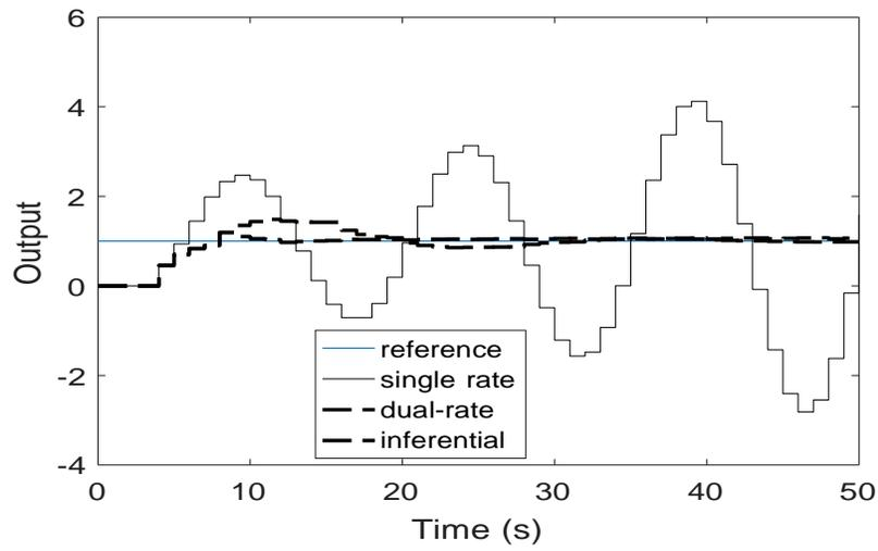
Figure 17: Example 2. Time response with MPM
