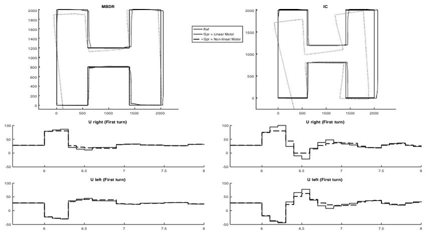
Figure 24: UGV. Linear and Non-linear servomotors comparison
