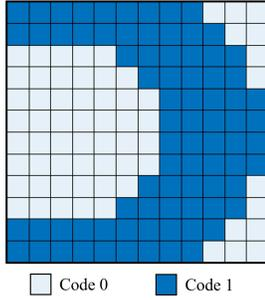
Fig. 10. Coding pattern of the passive RIS under vertical polarization.
