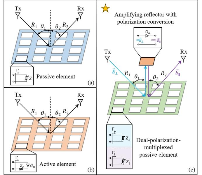
Fig. 1. Architectures of RISs. (a) The passive RIS. (b) The conventional distributed active RIS. (c) The proposed CA-RIS.
