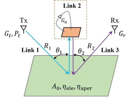
Fig. 2. Illustration of the CA-RIS energy flow links for path loss analysis.
