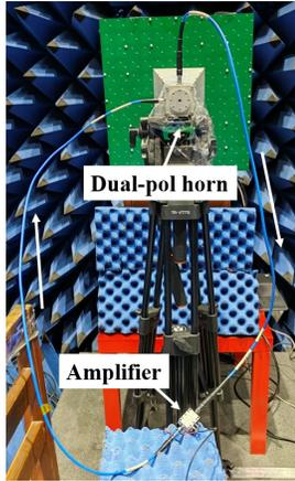
Fig. 3. Design of the amplifying reflector using an amplifier and a dual-polarized horn antenna.
