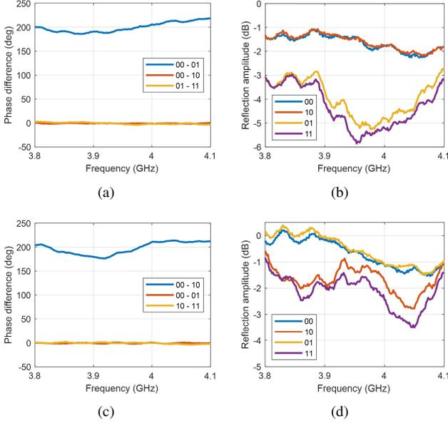
Fig. 6. Measurement results of the passive RIS. (a) Reflection phase differences under  $Pol_h$ . (b) Reflection amplitudes under  $Pol_h$ . (c) Reflection phase differences under  $Pol_v$ . (d) Reflection amplitudes under  $Pol_v$ .
