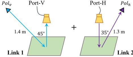
Fig. 12. Schematic of the two-step measurement.
