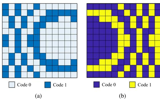
Fig. 8. Coding patterns of the CA-RIS. (a) Coding pattern for the vertical diodes, corresponding to the  $35^\circ$  incident wave. (b) Coding pattern for the horizontal diodes, corresponding to the  $45^\circ$  reflected wave.
