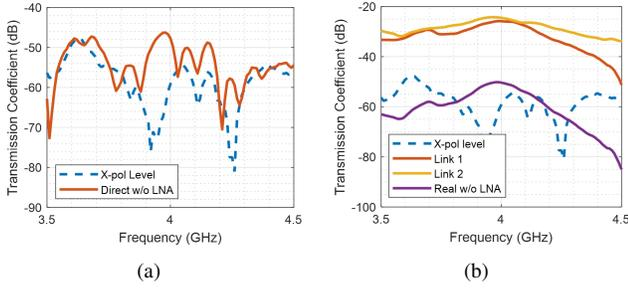
Fig. 11. The direct measured result and the two-step measured result. (a) Measured cross-polarization level of the system and the direct measured results based on the setup in Fig. 7(e)-(f). (b) Results based on the two-step measurement. The real path loss without LNA is obtained by summing two measured link losses, which is not affected by the cross polarization level.
