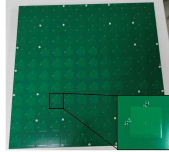
Fig. 5. Illustration of the dual-polarized passive 1-bit RIS prototype.
