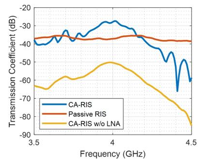
Fig. 9. Measured transmission coefficients of the CA-RIS, passive RIS and CA-RIS without LNA respectively.
