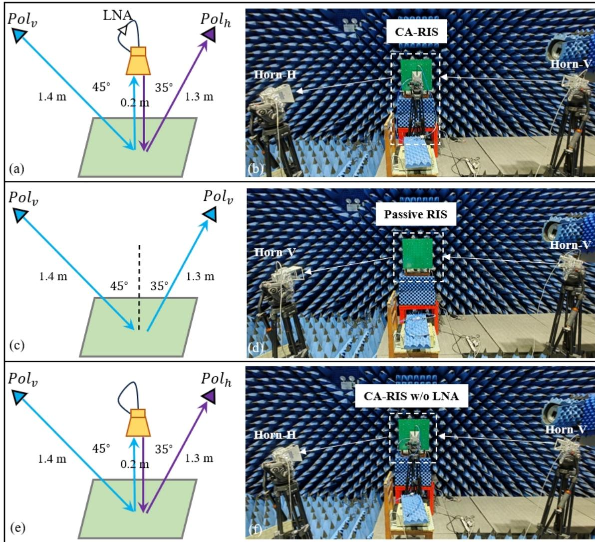
Fig. 7. Measurement schematics and setups of (a)-(b) the CA-RIS, (c)-(d) the passive RIS, and (e)-(f) the CA-RIS without the LNA.
