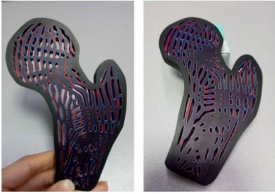
(a) Specimen of the optimized four-phase hip bone [8]
