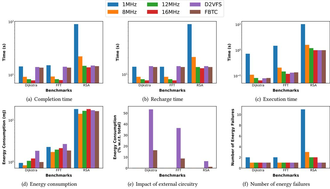
Fig. 19. Results with the energy-moderate source and Mementos with ADCMINV,  $C = 80\mu\text{F}$ , and  $V_{\text{boot}} = 3.6\text{V}$ .
