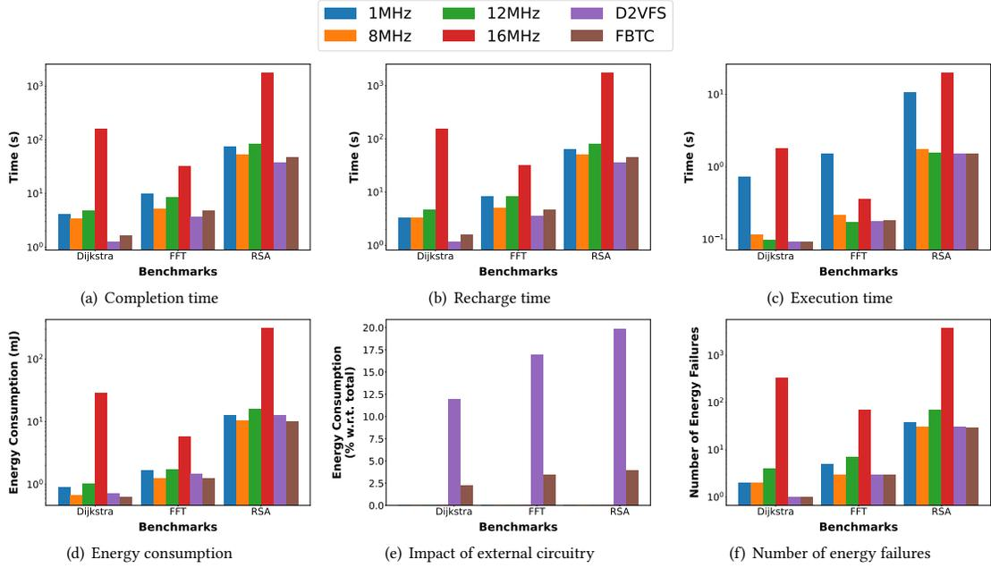
Fig. 22. Results with the energy-poor source and Mementos with ADCMINV,  $C = 80\mu\text{F}$ , and  $V_{\text{boot}} = 3.6\text{V}$ .
