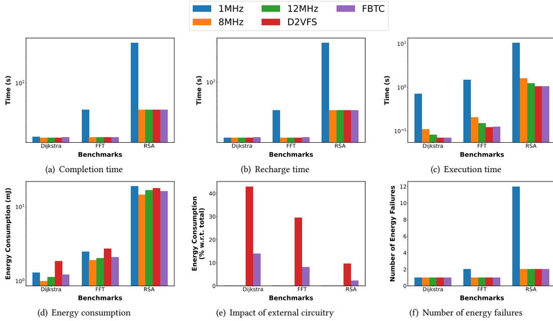
Fig. 20. Results with the energy-moderate source and Mementos with ADCMINV,  $C = 20\mu\text{F}$ , and  $V_{boot} = 3.6\text{V}$ .
