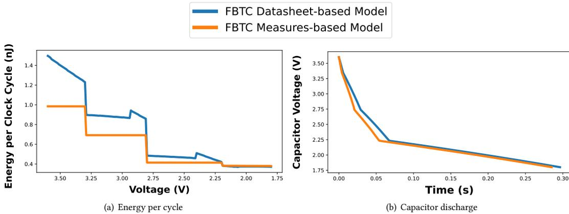
Fig. 14. Comparison of FBTC datasheet-based model against FBTC measures-based model.
