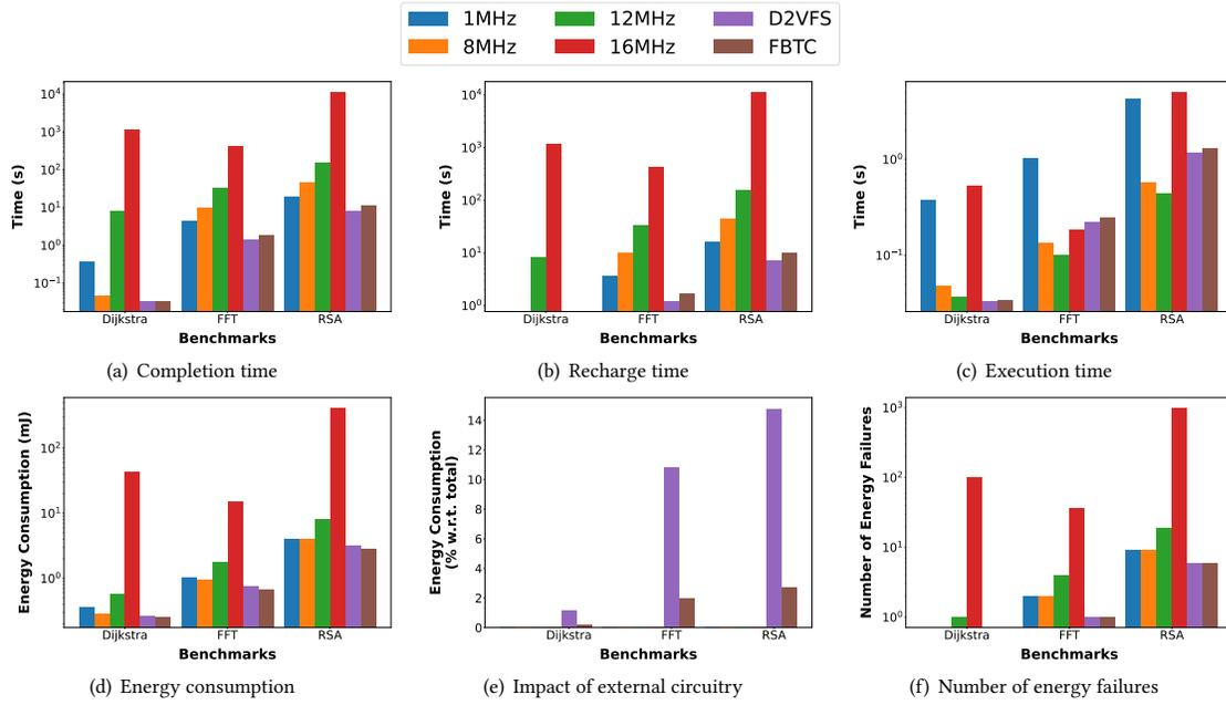
Fig. 21. Results with the energy-poor source and Hibernus,  $C = 80\mu F$ , and  $V_{boot} = 3.6V$ .
