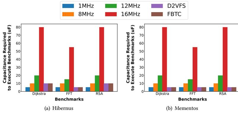
Fig. 12. Minimum capacitance required to execute benchmarks at a given frequency.
