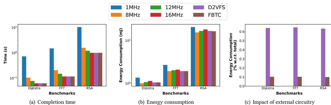
Fig. 16. Results with the energy-rich source and Mementos,  $C = 80\mu\text{F}$ , and  $V_{\text{boot}} = 3.6\text{V}$ .
