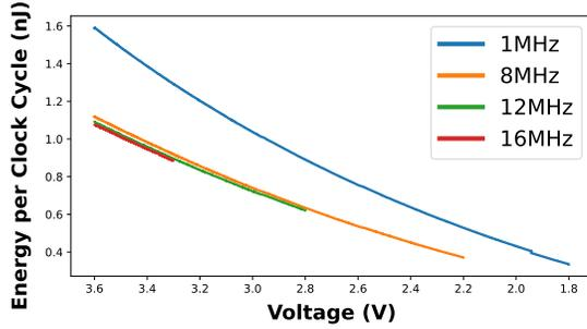
Fig. 2. Energy consumption per clock cycle at various voltage and frequency ranges for the MSP430-G2553 [4, 35].
