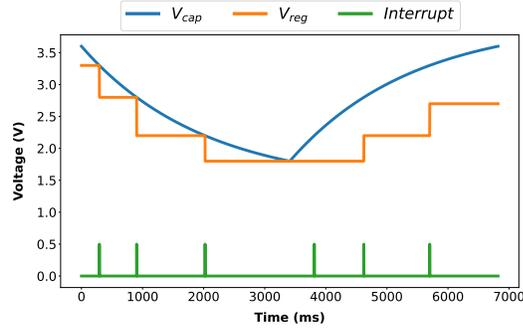
Fig. 7. Example of  $D^2VFS$  behavior.
