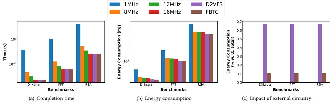
Fig. 15. Results with the energy-rich source and Hibernus,  $C = 80\mu\text{F}$ , and  $V_{\text{boot}} = 3.6\text{V}$ .
