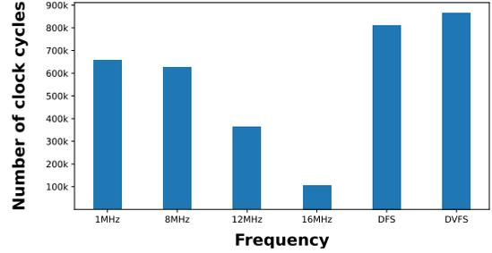
Fig. 3. Clock cycles executed in a single discharge from 3.6V of a  $100\mu F$  capacitor for various frequency configurations for the MSP430-G2553 [35].
