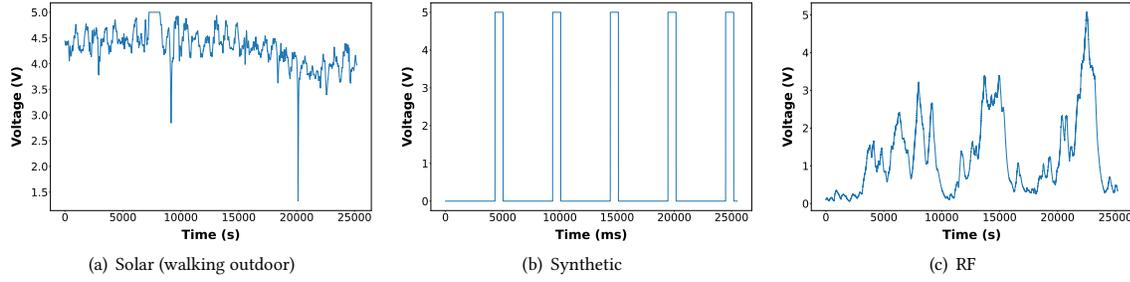
Fig. 11. Voltage traces of the considered energy sources.
