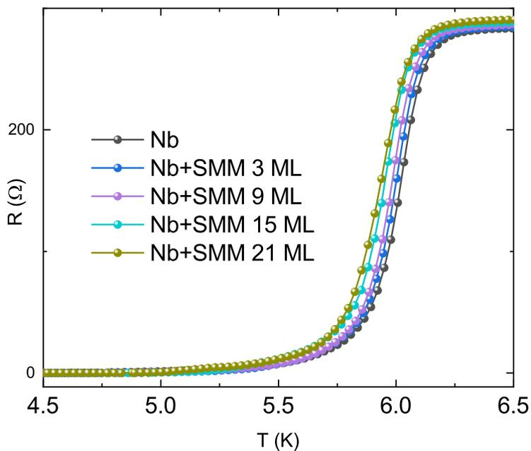
Figure S3: Temperature dependence of resistance of bare Nb track and Nb track with different layers of mixture of BA and SMM.
