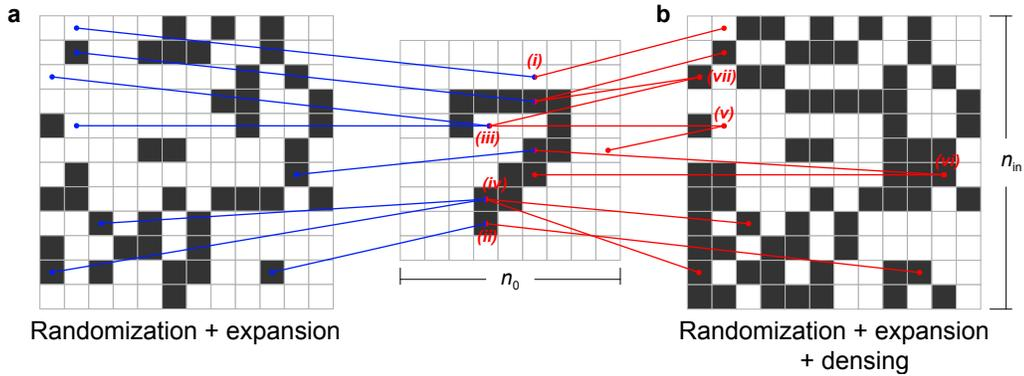
Figure 3: Schematic depicting the conversion of a binarized initial signal lattice of size  $n_0 \times n_0$  into an input signal lattice of size  $n_{\text{in}} \times n_{\text{in}}$ , utilizing randomization and expansion, both without (a) and with (b) signal densing.
