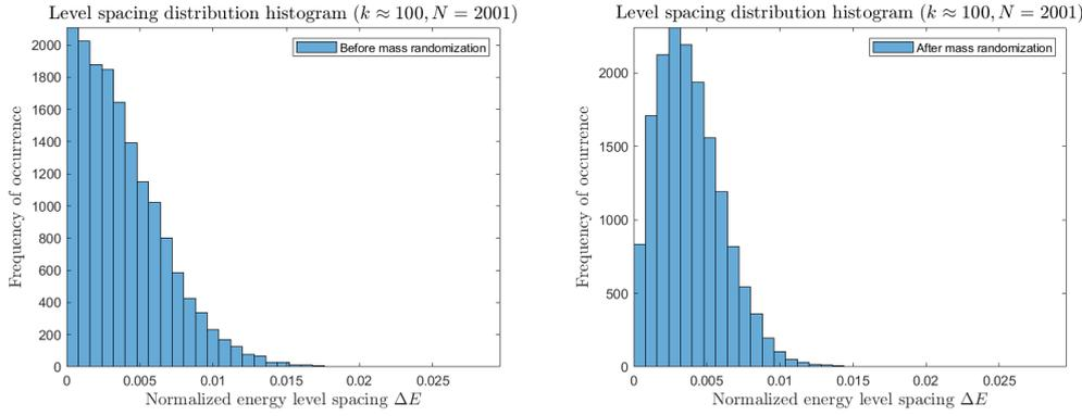
Figure 8: The level spacing distribution for  $k \simeq 100$ . It can be seen that due to degeneracies arising from symmetries or near-symmetries, the distribution does not match the GOE form (left panel). The distribution matches the GOE form after introducing a random small perturbation of  $10^{-3}m$  (right panel).
