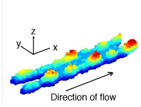
FIG. 8. Three dimensional biofilm growing on the bottom of the pipe.
