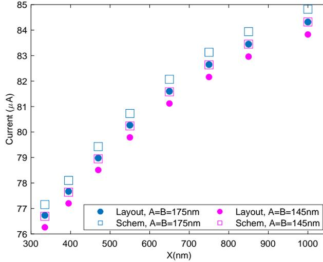
**Fig. 5:** Impact of layout-dependent effects on an LVT PMOS drain current in 65nm technology.
