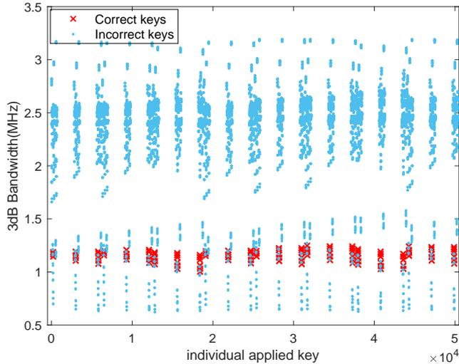
**Fig. 13:** Variation in the 3dB bandwidth of the OTA for the applied keys.
