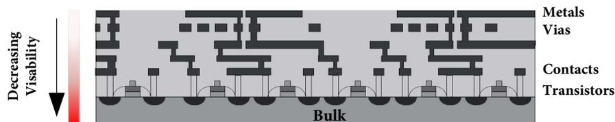
**Fig. 1:** Cross section of the metal stack in an IC. Moving towards the base layer, the visibility decreases and the effort to reverse engineer increases.
