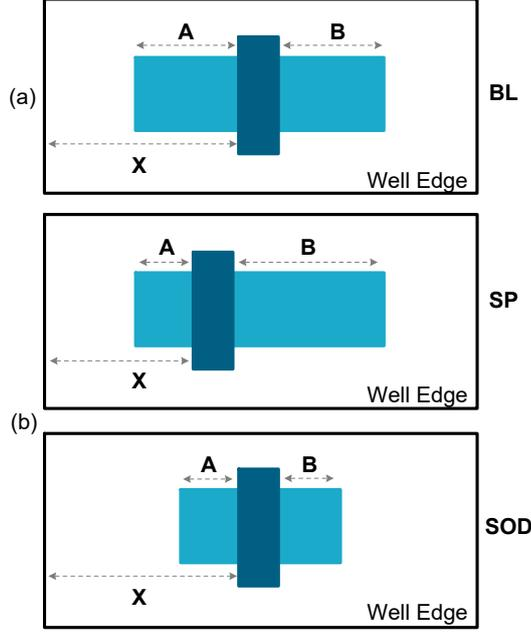
**Fig. 2:** Layout-dependent effects. (a) Simplified transistor layout, baseline. (b) Different transistor arrangements, used for obfuscating analog circuits. OD is the oxide diffusion, and PO is the poly (gate). A and B are the distances between the poly and the OD edges, and X is the distance between the poly and the well edges. X relates to WPE, and A and B relate to LOD.
