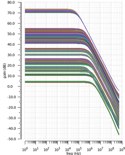
Fig. 15: Layout-based effects on the OTA simulated for 300K keys.
