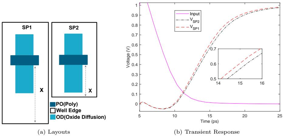
**Fig. 7:** Transistor layouts with different variants of the SP arrangement. The impact of WPEs on transient response of inverters with these layouts for PMOS transistors.
