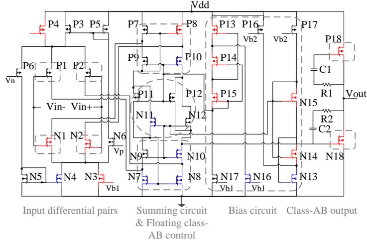
**Fig. 10:** Schematic of OTA circuit. Multiple subcircuits such as input differential pairs (P1, P2, N1, N2), summing circuit (P7-P10, N7-N10), bias circuit (P13-P17, N13-N17), and class-AB output (P18, N18) are used for applying the layout-based effects. Red, blue, and black transistors represent arrangements SOD, SP, and BL, respectively.
