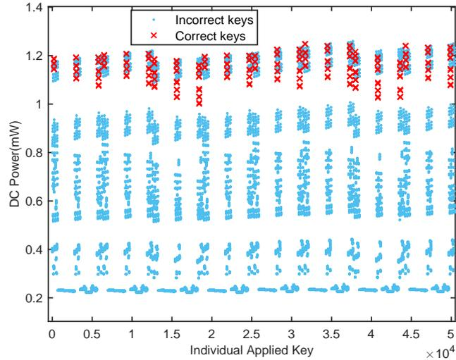
**Fig. 14:** DC power consumption for the applied keys.
