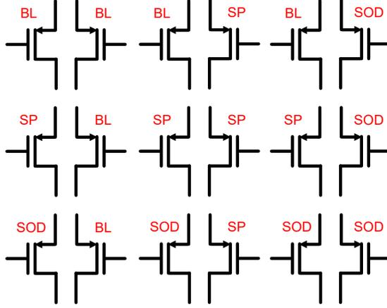
**Fig. 11:** Pairs of arrangements. One pair of arrangements in the based design can be hidden among a subset of 8 pairs of arrangements.
