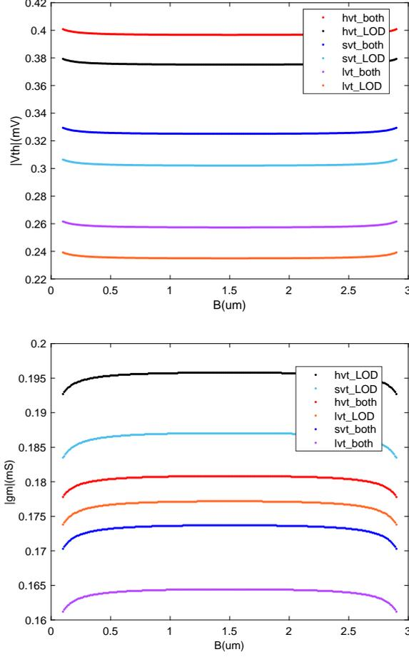
**Fig. 3:** Effects of LOD and both LOD and WPE on the absolute values of voltage threshold and transconductance of PMOS transistors with a minimum length and representative width.  $B$  is shown in Figure 2.
