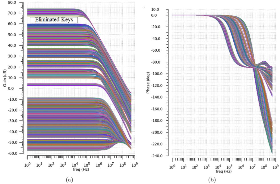
**Fig. 12:** Layout-based effects on (a) the OTA gain and (b) phase simulated for 50K keys. The gap marked in the graph is the result of purposefully removing nearly correct keys.
