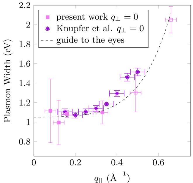
FIG. 5. Plasmon width at half maximum in dependence on the momentum transfer parallel to the layers at  $q_{\perp} = 0$ . For comparison the corresponding data from a Drude fit of our previous EELS measurements reported in Ref. [36] was added as dark purple stars. The excitations in the continuum range are marked by open symbols.
