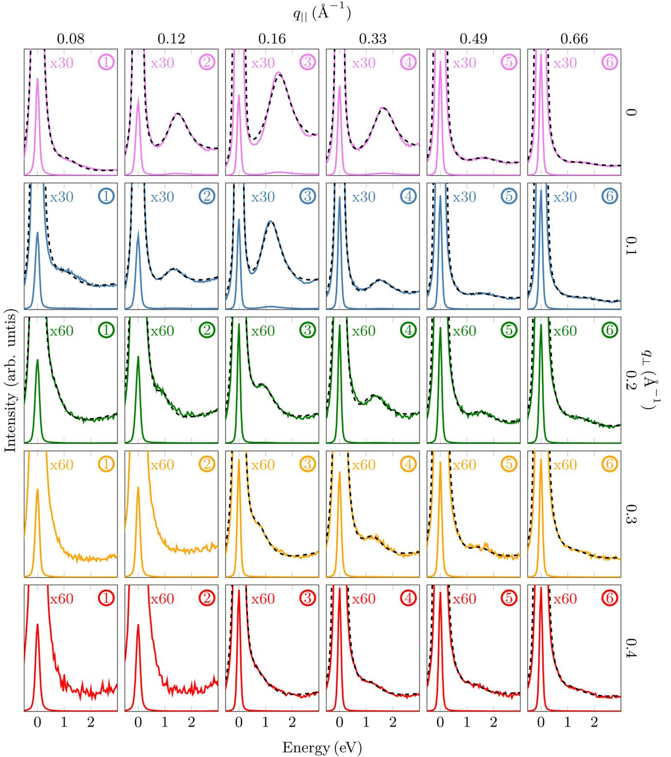
FIG. 3. Electron energy-loss intensities for various  $q_{||}$  and  $q_{\perp}$  values. The indicated numbers (1-6) and the colors correspond to the momentum values depicted in Fig. 2. Experimental spectra are depicted twice (normal scale + 30x/60x scaled up) to show both the zero loss peak and the plasmon peak. The black dashed lines correspond to fits of a superposition of a Voigt profile (zero loss), a Drude function (plasmons), and a background (see Methods).
