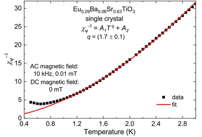
FIG. 8. Temperature dependence of inverse AC magnetic susceptibility  $\chi_{\psi}^{-1}$  measured in zero DC magnetic field on the EBSTO single crystal. The data of  $\chi_{\psi}^{-1}(T)$  (obtained by normalizing the data of AC  $\chi_{\psi}(T)$  from Figure S10 to the DC  $\chi_{\psi}(T)$ ) follow the power-law dependence with parameters  $A_1 = (4.8 \pm 0.2) \text{K}^{-q}$ ,  $A_2 = (0.2 \pm 0.2)$ ,  $q = (1.7 \pm 0.1)$  in the temperature range 1 – 3 K.
