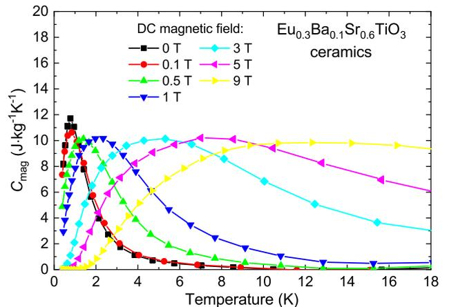
FIG. 6. Temperature dependence of the magnetic contribution to heat capacity measured in various DC magnetic fields on the  $\text{Eu}_{0.3}\text{Ba}_{0.1}\text{Sr}_{0.6}\text{TiO}_3$  ceramics.
