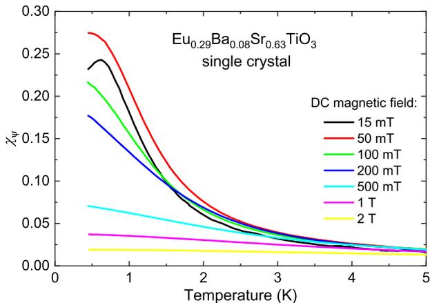
FIG. 4. Temperature dependence of magnetic susceptibility measured in various DC magnetic fields on the EBSTO single crystal. The decrease of  $\chi_{\psi}$  with increasing magnetic field is a consequence of gradual saturation of magnetization (see also Fig. S13 in Supplemental material[34]). At low temperatures, this effect is significant even for weak magnetic fields.
