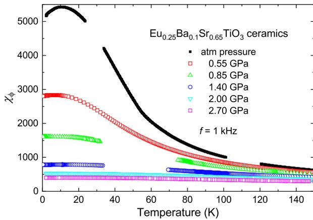
FIG. 3. Temperature dependence of the 1 kHz dielectric susceptibility measured at various hydrostatic pressures on the  $\text{Eu}_{0.25}\text{Ba}_{0.1}\text{Sr}_{0.65}\text{TiO}_3$  ceramics.
