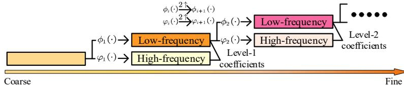
**Fig. 3.** The process of SWT decomposition. Here the low-pass and high-pass filters  $\phi(\cdot)$  and  $\varphi(\cdot)$  are upsampled after each level of decomposition.
