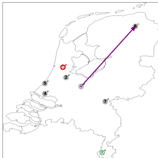
Figure 1: (Figure best viewed in color.) Visualization of the K -DTMPA model for an asset network of M = 8 machines serviced by K = 3 maintenance engineer. Blue dots on top of machine nodes indicate that the machine is healthy, orange when alerted or red when the machine is down. The engineers are colored cyan, green and purple and are located at Amsterdam, Maastricht and Utrecht, respectively. At discrete decision epochs, engineers can either: (i) idle/continue, (ii) travel to another location or (iii) start maintenance at the current location.
