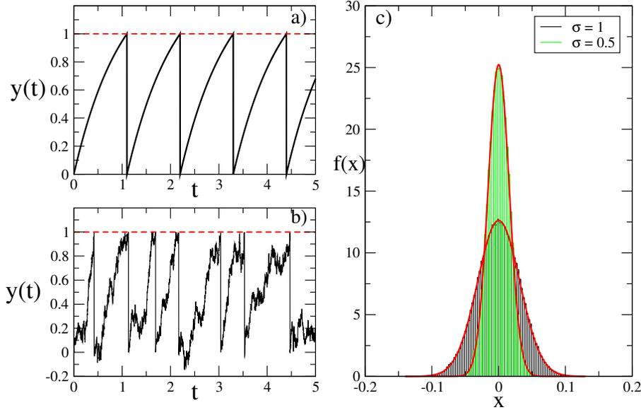
Figure 2: (a)-(b) Time series of noise-free ( $\sigma = 0$ ) and noisy trajectory ( $\sigma = 0.5$ ) for LIF neuron (see Eqs. (5)-(6)) with a fixed  $a = 1.5$ . When the membrane potential  $y(t)$  hits the threshold 1 (red dashed line), it is reset to 0. (c) The probability density for white noise when  $\sigma = 0.5$  (green) and  $\sigma = 1$  (black) generated from the simulation. The solid red curves correspond to  $f(x)$  in the Equation 10.
