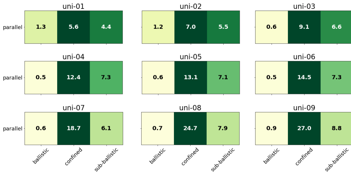
Figure 17: Average values of contact duration t_c for unidirectional flow scenarios.
