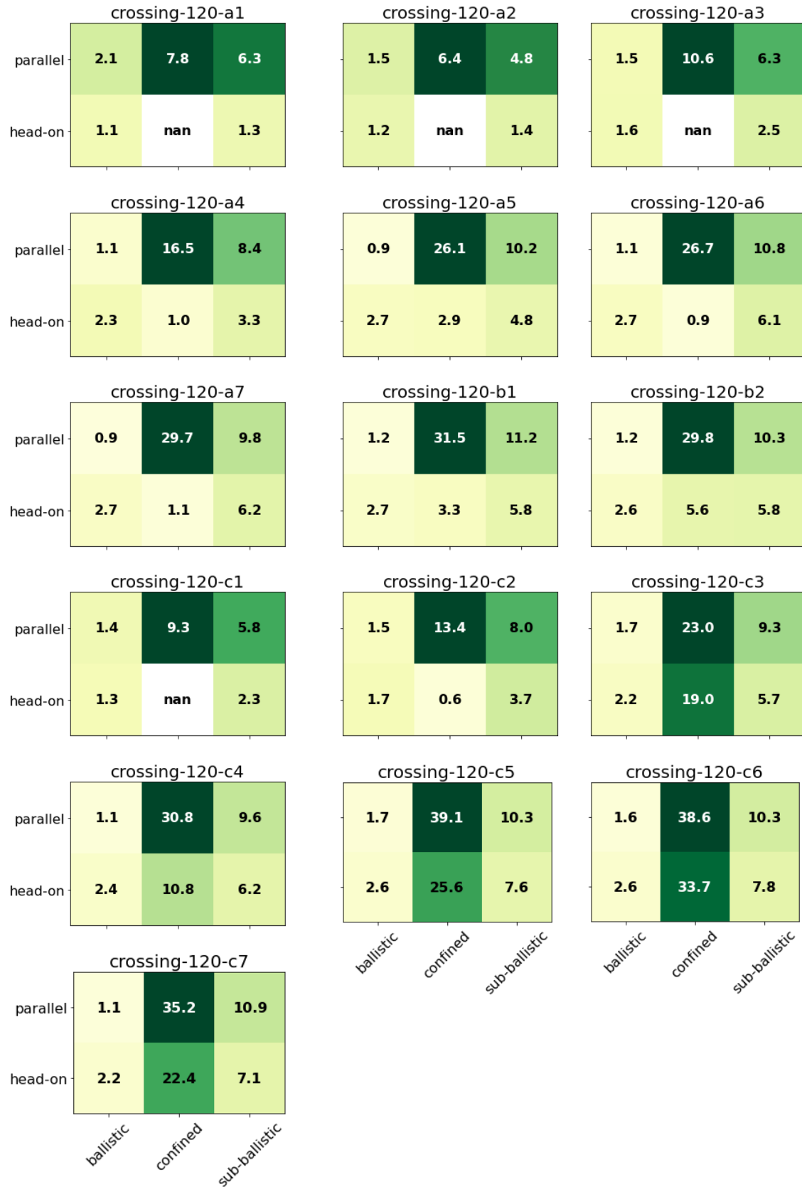
Figure 20: Average values of contact duration t_c for 3-way crossing flow scenarios.
