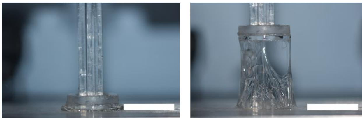
**Figure S16.** Broken adhesive after a probe-pull experiment. The scale bar is 2 cm.
