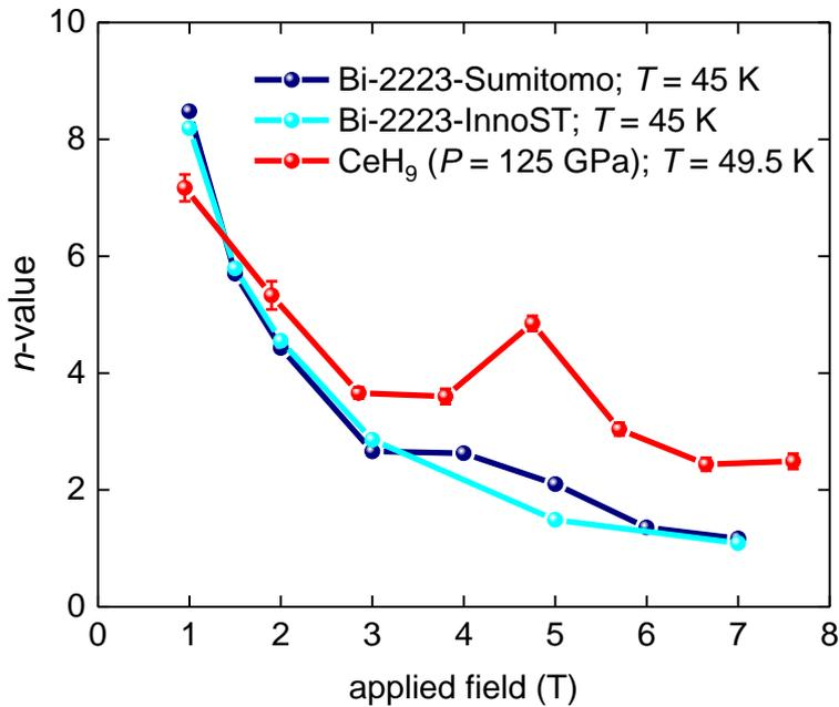
**Figure 3.** Field dependence of  $N$ -values for 1G-HTS wires (data by Wimbush and Strickland [29]) and CeH<sub>9</sub> ( $P = 125$  GPa) (raw  $V(I)$  datasets reported by Semenok *et al* [15]).
