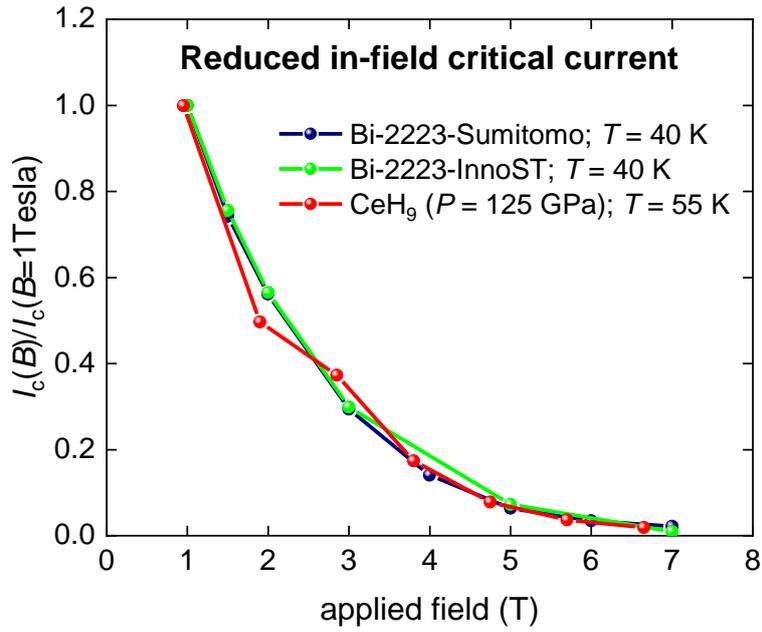
**Figure 2.** Reduced transport in-field critical currents (defined by  $E_c = 1 \mu\text{V}/\text{cm}$  criterion) for polycrystalline superconductors. Blue – Sumitomo 1G-HTS wire (data by Wimbush and Strickland [29]). Green – InnoST 1G-HTS wire (data by Wimbush and Strickland [29]). Red - CeH<sub>9</sub> ( $P = 125$  GPa), raw  $V(I)$  datasets reported by Semenok *et al* [15] in their Figure S6.
