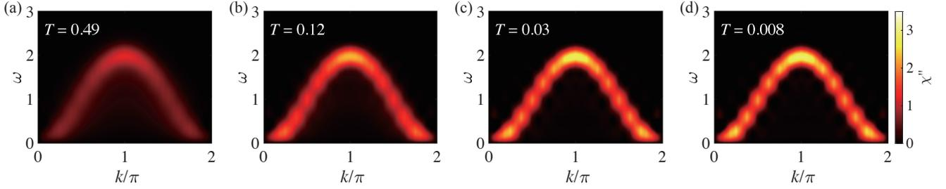
FIG. S6. Contour plot of spectral density  $\chi''$  of a pure FM Heisenberg chain with  $L = 16$  at various temperatures.
