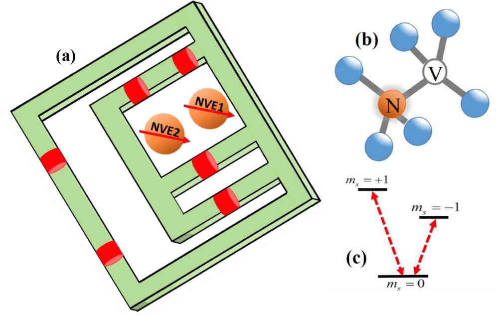
Figure 3: (a) Two ensembles of NV centers coupled to a superconducting flux qubit consisting of four Josephson junctions forming the main loop and an  $\alpha$  loop. (b,c) Crystal-lattice (b) and energy (c) diagrams of an NV center in diamond.
