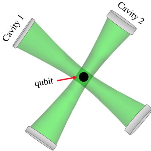
Figure 1: A scheme of the generating N00N state. The system consists of two cavities interacting with a qubit. The qubit dispersively interacts with the cavities.
