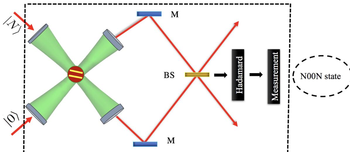
Figure 4: Architecture of the entangled state generation setup. The input state first interacts with the system of the two resonators interacting with a qubit for as long as  $\kappa t = \pi/4$ . Then the photons in the resonators are sent to a beam splitter. Finally, by applying a Hadamard gate and performing a measurement on the qubit we attain a N00N state.
