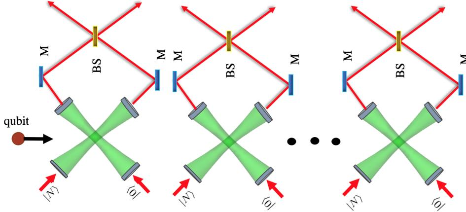
Figure 5: The network of multi-N00N state generation architecture. The qubit is sent through the resonator network to interact with each resonator pair. Then the photons inside the each pair is sent to a beam splitter.
