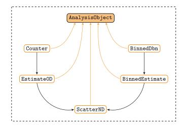
Figure 4: User-facing class inheritance structure in YODA 2. The orange lines show that all these types inherit from the persistency and metadata features of AnalysisObject, and the black arrows indicate the direction of live-to-inert type-reductions. Direct type reductions to ScatterND from Counter and BinnedDbn are also allowed, bypassing the intermediate Estimates.
