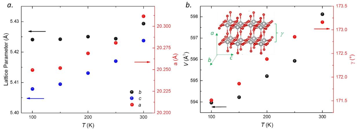
**Fig. 2. a. Temperature-dependent lattice parameters and Ni-O-Ni bond angle.** Temperature-dependent lattice parameters ( $a$ : red symbols on the right axis,  $b$  and  $c$ : black and blue symbols, respectively, on the left axis) in  $Cmcm$  Sr-doped  $\text{La}_3\text{Ni}_2\text{O}_7$ . **b.** temperature-dependent volume of the unit cell (black symbols on the left axis) and the out-of-plane angle of Ni-O-Ni,  $\gamma$ , as indicated in the inset (red symbols on the right axis).
