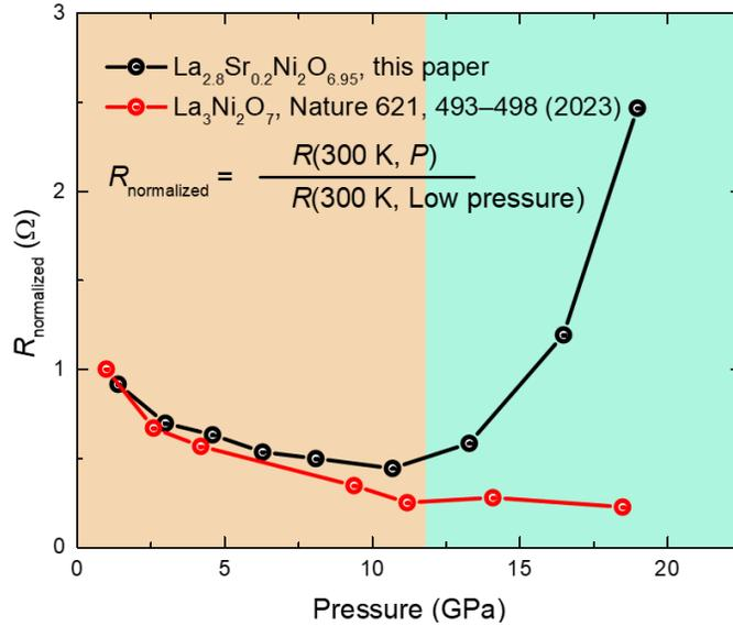
**Fig. 4. Comparison of pressure dependent normalized resistance at 300 K.** The resistance at 300 K is normalized with the first low pressure data by forcing the first data point to line on the extrapolated trend. The data of this paper is given in black, and the data from the reference is given in red. The color edge between pink and green indicates the start of structure transition and superconducting transition in  $\text{La}_3\text{Ni}_2\text{O}_7$ .
