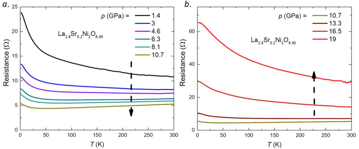
**Fig. 3. Temperature-dependent electrical resistance from 2 K to 300 K at pressures up to 19 GPa. *a.* Pressure ranges from 1.4 - 10.7 GPa showing the insulator to metal trend as the pressure increases (dashed arrow pointing down). *b.* Pressure ranges from 10.7 - 19 GPa showing the metal to insulator trend as the pressure increases (dashed arrow pointing up).**
