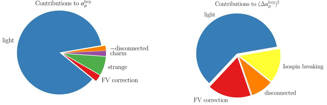
**Figure 2:** Contributions to the value (left) and the squared uncertainty (right) of  $a_\mu^{\text{hvp}}$  based on the calculation in [30]. The quark-disconnected contribution is negative.
